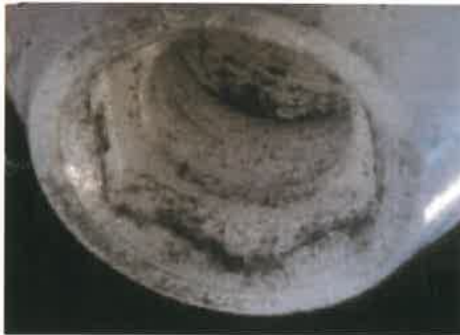
Figure 25. Photograph of the apical end of the CerAdapt abutment from the implant in Figure 23. Note the black material on the internal hex of the CerAdapt abutment. These debris are titanium filings that have been abraded from the external hex of the titanium implant.
