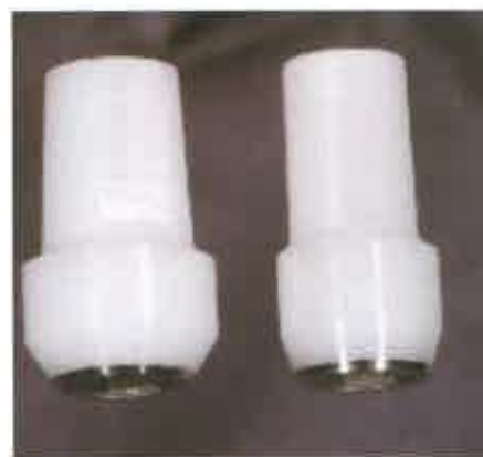
Figure 1. ZiReal Posts for the 4.1-mm implant restorative platforms with two different diameters (5 mm and 6 mm). Zirconia is fused to titanium inserts at the apical end of the abutments providing for a metal-to-metal interface between the zirconia abutments and the titanium implants.
